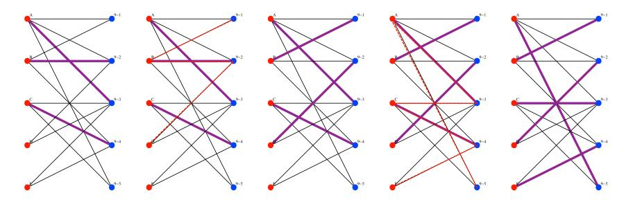
Given M,  $P = D \rightarrow 9-2 \rightarrow B \rightarrow 9-1$  is an M-augmenting path. Toggling the edges in P gives a new matching M'.
